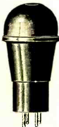
Shielded 201A Tube, entirely covered with Bakelite shield—does a way with micro-phonous noises.
